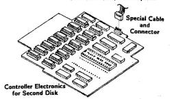
You can have this useful Controller plug-in alone or as an option to any jrHOTSHOT Fast Memory. Either way, this makes it easy to add a second floppy drive to your PCjr. No additional power supply is needed for this plug-in. We can suggest several economical sources, such as True Data Products (800)-635-0300, that have the external floppy drive housed in a case with power supply for the drive.
